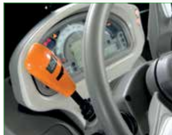
WET CLUTCH WITH SENSE CLUTCH SHUTTLE MODULATION CONTROL ALLOWING SMOOTH DIRECTIONAL CHANGES
