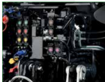
120 L/MIN CAPACITY CLOSED-CENTRE HYDRAULIC SYSTEM
