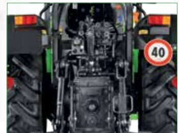
POWERFUL HYDRAULIC SYSTEM WITH A CAPACITY OF UP TO 60 L / MIN
