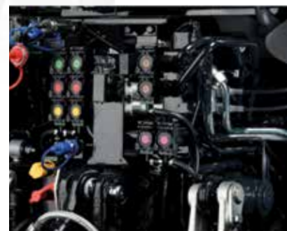
Hydraulics. 120 L/min capacity closed- centre hydraulic system
