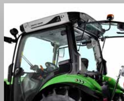
Suspended cab with CAT 4 cab filtration system
