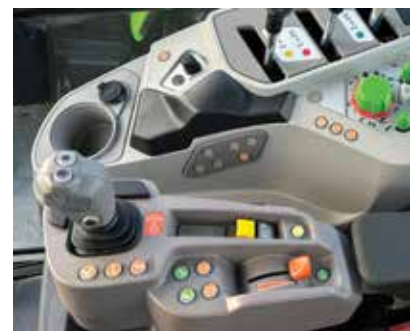
20 speed electronic armrest controlled full powershift transmission
