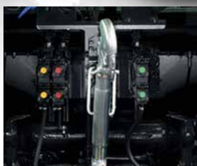
RC models feature closed centre hydraulics with 120l/min flow rate
