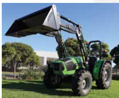
Agrolift 2940 CRX Loader Lift height up to 2.7 metres
