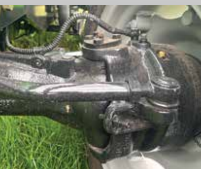
Oil-immersed disc brakes on all four wheels
