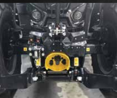
Front linkage and PTO standard on the Warrior 6230
