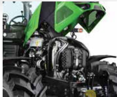
Tier 3 FARMotion Engine 4-cylinder turbo intercooled
