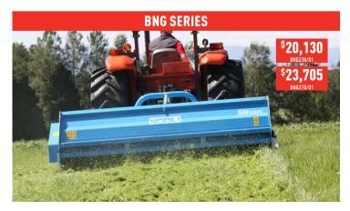
The Nobili BNG series are fitted with a tailboard that can be opened for ease of maintenance and a mulching bar to produce a finer mulch.
