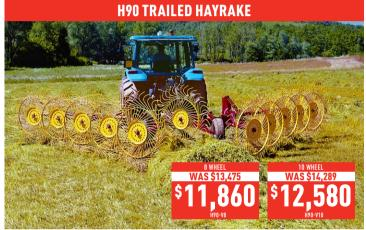
Suitable for raking, turning and spreading hay crops and grain crop stubble. 8 and 10 wheel models with working widths of 6.1 and 7m respectively Single set hydraulics via tractor remote
