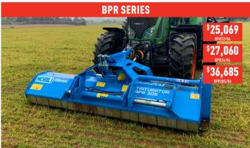
The Nobili reversible BPR series mulchers are multi-purpose machines ideal for pasture topping with a double hitch that fits to the front or rear of the tractor and hydraulic side shift. Suited to tractors up to 175HP with cutting height maintained by rear roller.
