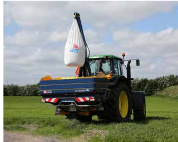
BXL 1300 can lift up to 1300 Kg and can be fitted on spreaders up to 3300 litres.
