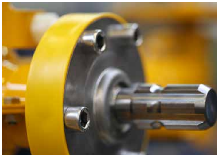
The integrated waterproof and maintenance free overload clutch, protects against damage on the tractor, the PTO-shaft and the transmission in case of PTO-start at high tractor revs.
