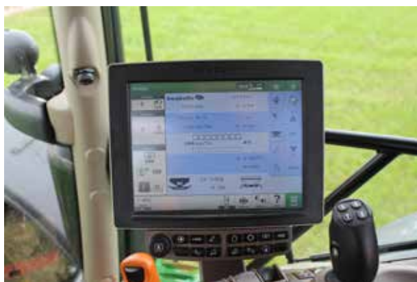
On speed independent spreaders, the PTO-revolutions are monitored directly on the display.
